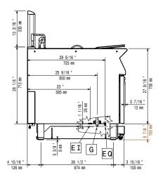
ΕI Electrical inlet (power) EQ Equipotential screw Gas connection
